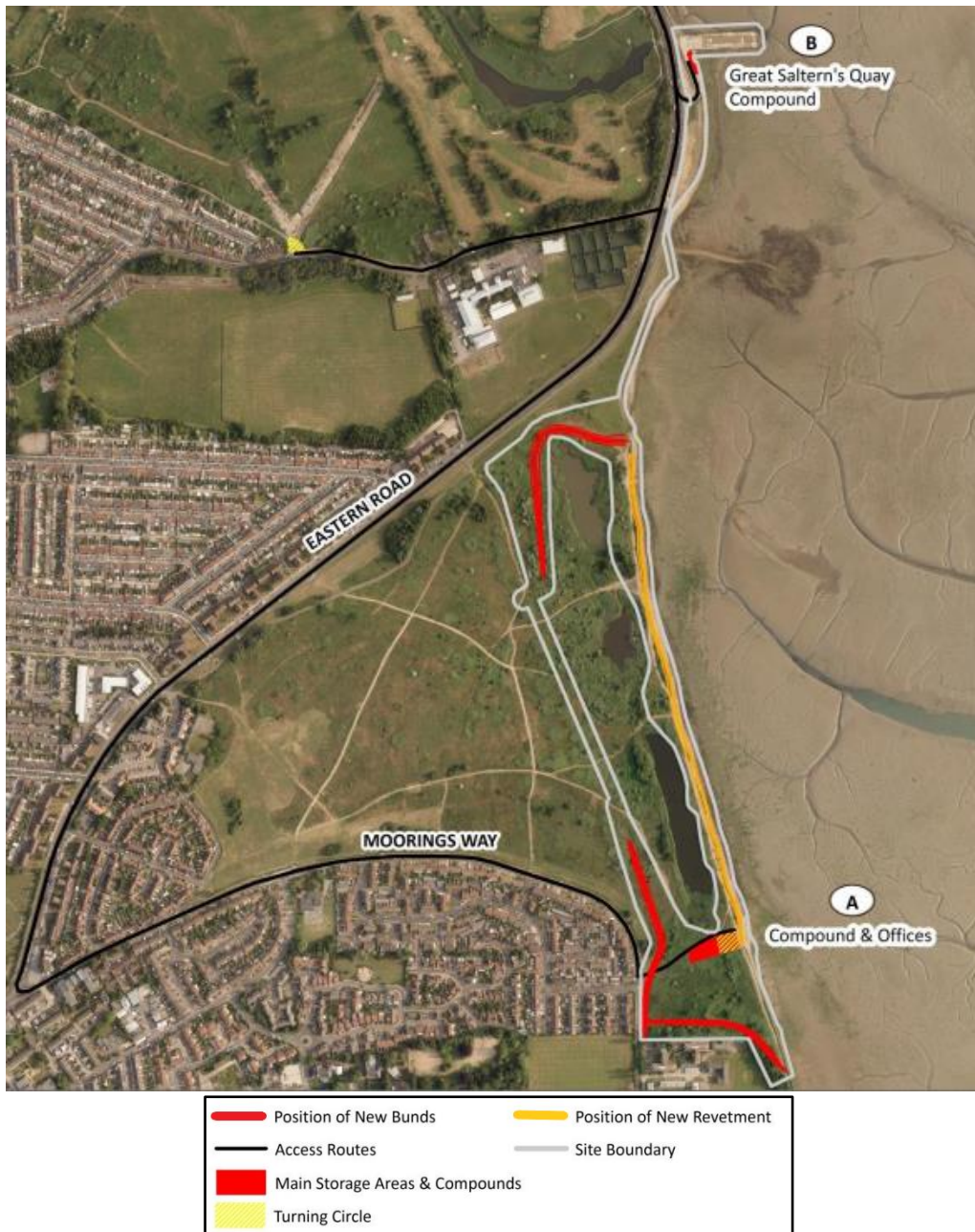
Figure 7: Works comprising Phase 2 of the NPI Coastal Defence Scheme (Source: Coastal Partners)
